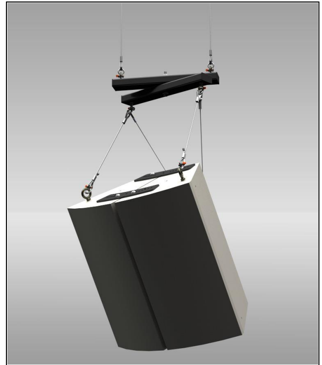
3 Point suspension using adjustable tilt Cable Kit, bridle at the rear and SAS-1WA-20 One way Array Rigging System
