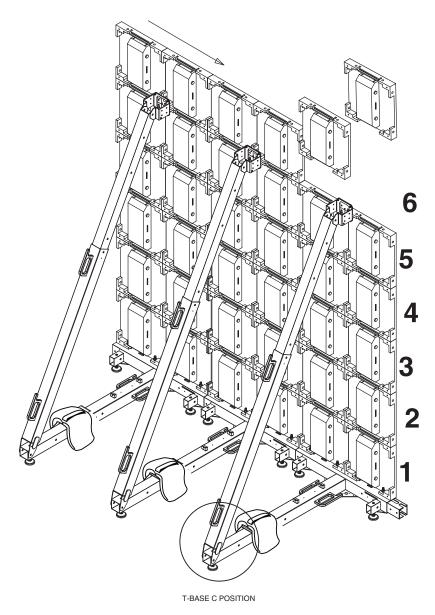
ASSEMBLE THE **SEVENTH TIER TO THE SIXTH TIER**. IF THE VIDEO WALL WILL GROW HIGHER THEN RAISE THE HEIGHT OF THE BACK BRACE, ONE BY ONE, TO THE NEXT HIGHER POSITION AS TILES ARE BEING ADDED. THE T-BASE EXTENSIONS MUST ALREADY BE ADJUSTED OUT TO THE C POSITION UNLESS A SOUND STRAPPING METHOD IS EMPLOYED IN PLACE OF BALLAST.
