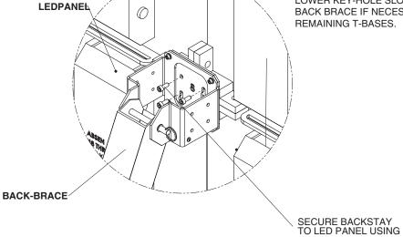
ASSEMBLE THE **FIFTH TIER** AND SECURE THE TILES LOWER CORNER SCREWS TO THE UPPER HOLES OF THE BACK STAY. LOCK INTO PLACE WITH THE FOURTH SCREW IN THE NON-SLOTTED SCREW HOLE.
