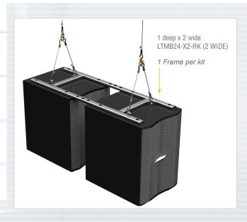
Unique attributes of the Bose MB24 low frequency sub woofer require specific interdependent physical relationships when arraying these cabinets together. ATM Fly-Ware's LTMB24 overhead truss system is an efficient lightweight suspension frame that places these cabinets into their acoustically correct horizontal position and allows them to be aimed and suspended as one structure, two-wide, quickly and easily.
