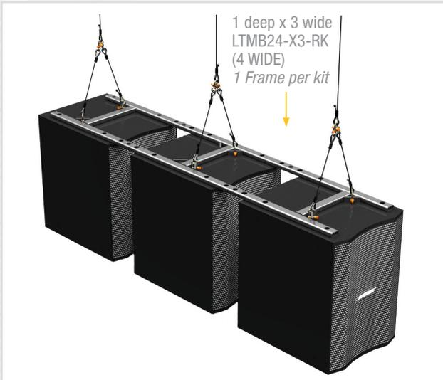
Unique attributes of the Bose MB24 low frequency sub woofer require specific interdependent physical relationships when arraying these cabinets together. ATM Fly-Ware's LTMB24 overhead truss system is an efficient light-weight suspension frame that places these cabinets into their acoustically correct horizontal position and allows them to be aimed and suspended as one structure, two-wide, quickly and easily.
