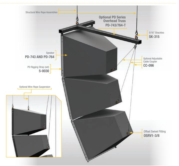
WARNING: Mounting and/or suspension of loudspeakers requires experienced professionals. Improperly installed loudspeakers can result in property damage, personal injury and/or liability to the installing contractor.
