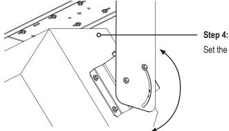
Set the desired tilt angle of the speaker and permanently tighten the side bolts.
