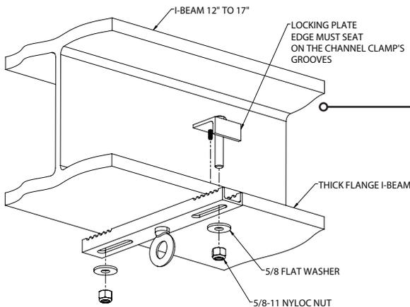
The BC7-12 channel style beam clamp to provide a load rated overhead rigging point from structural I-Beams with flange widths ranging between 7" and 12" and with 1/4" to 1" thick flanges. This beam clamp model provides a fast, easy and safe way to rig direct loads, bridles and hitches from overhead.
