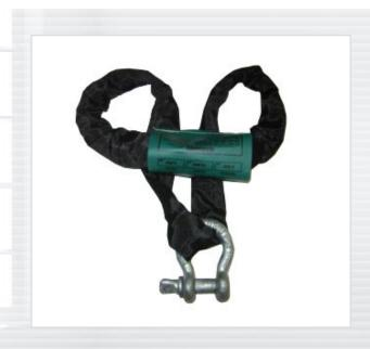
Steel band round slings are for the quick connection and temporary use of suspending objects from overhead lighting truss, structural beams, etc. Its internal cord is comprised of multiple wire rope bands, which lends itself for fire rated installations that may remain installed for long periods of time. Its soft external cover protects the finish of suspended surfaces and its black color lends itself ideally to
