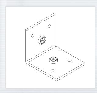
The CB Series internal braces secure cabinet panels together to serve as a mechanical back up to the joinery in woodworking. They anchor to the panels by way of flat head screws and also serve as an internal support for suspension hardware such as eyebolts, OSR fittings and single stud anchor plates.
