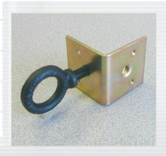
This Internal Brace provides a quick, simple and inexpensive way of providing fly point attachments to loudspeaker cabinets while adding cabinet integrity by securing the panels to each other.
