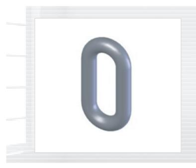
Weldless endlinks are produced from a single piece of metal eliminating the possibility of weld failure. This high strength load-rated link is ideal for use in coupling multiple span sections together, such as wire rope and rigging cha" Multiple sections of wire rope and rigging chain link together, using shackles. Its oval shape is designed for in-line use and is not to be side loaded.
