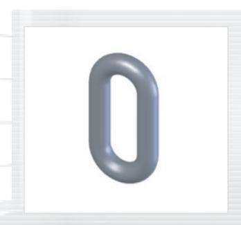
Weldless endlinks are produced from a single piece of metal so there is no chance for weld failure. This high strength load-rated link is ideal for use in coupling multiple span sections together, such as wire rope and rigging chain. Multiple sections of wire rope and rigging chain link together, using shackles. Its oval shape is designed for in-line use and is not to be side loaded.
