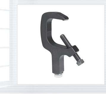
The MC-020-BT is created from high tensile, aircraft grade, extruded aluminum; so it's both stronger and lighter than cast iron clamps. The MC-020-BT's safety factor far exceeds industry standards, breaking at over 2-1/2 tons at an independent testing laboratory. It is half the weight and twice as strong as most cast iron clamps.
