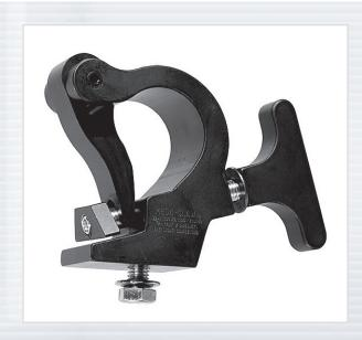
Adaptive's MC-025 Truss Clamp makes suspending items from truss and pipe fixtures safe and quick. Simply flip the link up, place clamp over the pipe and the MC-025 holds the weight of the fixture for you while you secure it with the solid 3/4" thick handle. The MC-025 will fit onto (1-1/2" Pipe) 1.9" OD to 2" OD.
