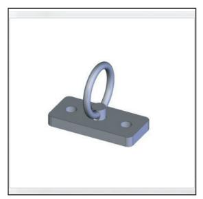
The OSRV2-1/2" offset swivel ring fitting mounts to flat surfaces, such as wood, steel and concrete. Secure with grade 8 fasteners (or equivalent) to their proper torque value. One 2" long 3/8 hex bolt is included for use with loudspeaker cabinets.
