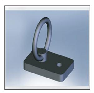
The OSRV1-3/8" offset swivel ring fitting mounts to flat surfaces, such as wood, steel and concrete. Secure with grade 8 fasteners (or equivalent) to their proper torque value. One 2" long 3/8 hex bolt is included for use with loudspeaker cabinets. M10X50mm hex bolts may be ordered separately.
