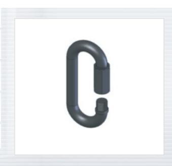
QuickLinks join two closed-end items together, such as wire rope assemblies, turnbuckles and eyebolts quickly and easily. They offer significant working loads for their size and serve as convenient coupling devices for temporary installations but, because its side locking turn style has the potential to loosen over time, QuickLinks are not recommended for overhead use.
