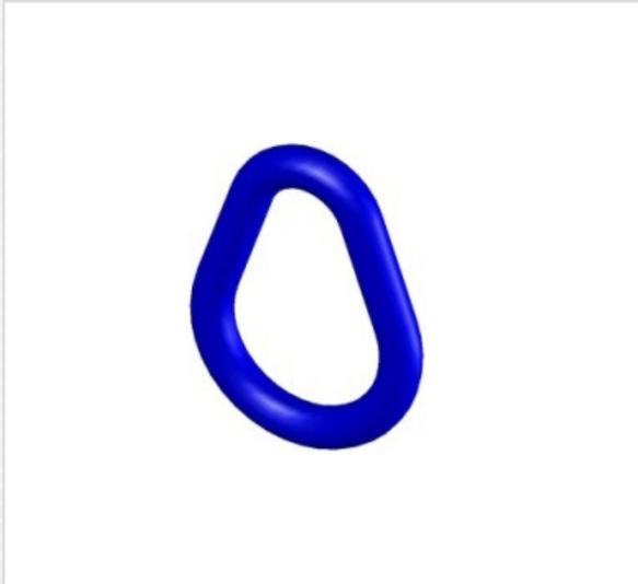
Weldless sling links are produced from a single piece of metal so there is no chance for weld failure. This high strength load-rated link is ideal for use in bridling two points (from the wider end), at angles from a third point (at the narrower end), such as with shackles or wire rope assemblies.
