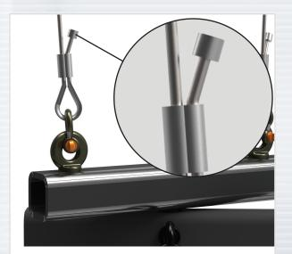
Wire rope stops are used to seal the end of a wire rope to prevent sharp frayed ends. Also called button stops, these aluminum cable stops are swaged on wire rope to cap the ends. Stop buttons should not be used for load bearing applications. Use with aluminum sleeves on galvanized wire rope.
