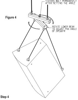
Tighten the  $\frac{1}{2}$ " x 5.5" long bolt permanently to set the pan angle of the speaker.
