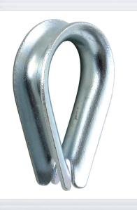
When a wire rope is terminated with a loop, a steel thimble is inserted in the eye to keep the rope from bending at too small of radius and damaging the rope. Thimble eyes also protect the wire rope from direct contact of other hardware and reducing wear and tear on the wire rope.
