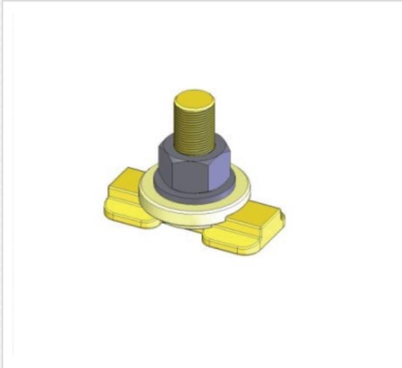
Loudspeaker cabinets equipped with L-track can be suspended with single and double stud fittings. The thread adapter, however, allows objects to be bolted to the cabinet, such as with AMFS truss modules by ATM FlyWare. Simply lock the threaded fittings into the L-track then fit the truss module over the studs and secure with the included locking style nuts.
