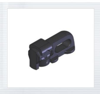
The double stud with ring option allows loudspeakers and other objects, equipped with L-track, to be secured from a wide range of readily available coupling devices such as, carabiners, quick links and shackles. This design does not offer a redundant locking feature that is sometimes required in overhead applications.
